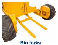
Hydraulically operated from the cage. A set of bin forks allow the operator to carry and shift bins in the row efficiently. Forks are easy to pin on and off. These forks have a maximum lifting capacity of 600kg.
